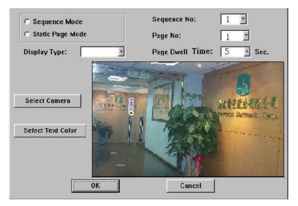
Please select Sequence Mode or Static Page Mode first. For Sequence Mode, you may select the Sequence No, then set the Page Dwell Time, Cameras, and Text Colors for each Page; for Static Page Mode, you may set the Cameras and Text Colors for each Display Type. To Select Camera or Select Text Color for a specific video window, please click on Select Camera button or Select Text Color button first, then click on the video window, the Camera number or Text Color will change accordingly.
